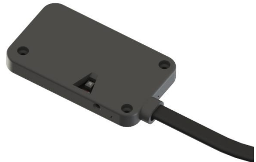
Fig. II: Server Tag backside with Temperature & humidity sensor
